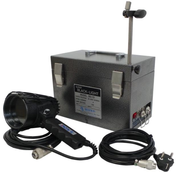
A BLACK LIGHT BD-70 is a U/V illumination light and is device used for searching for flaw of the Object to be tested by using light emission feature of fluorescent substance when performing the Magnetic particle flaw detection test or color check test.
